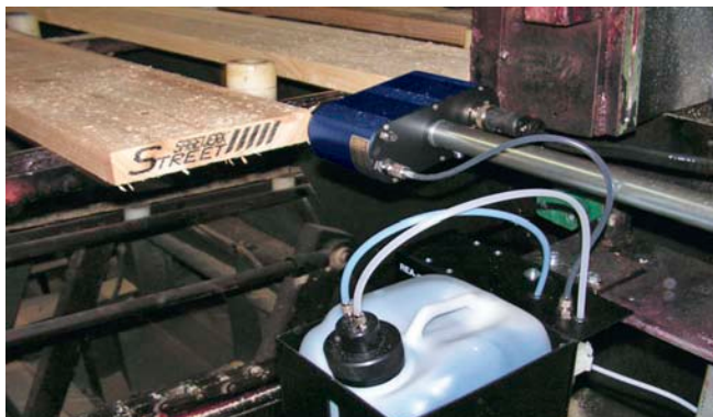
Marking on rough sawn timber boards
