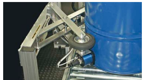
Barrel turning device
