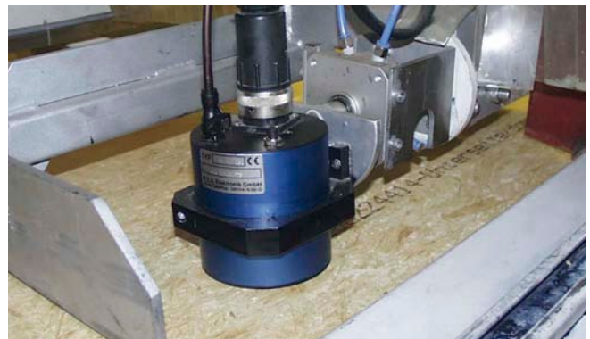
Coding of plywood boards
