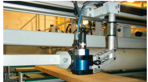
Vertical distance levelling device
