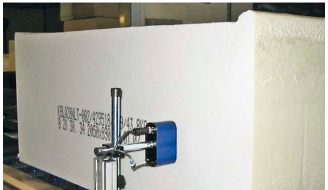
Marking of styrofoam blocks
