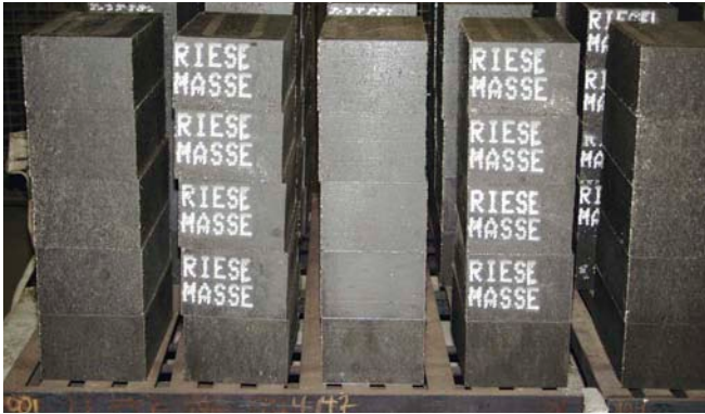
Refractory stone marking with high-temperature ink
