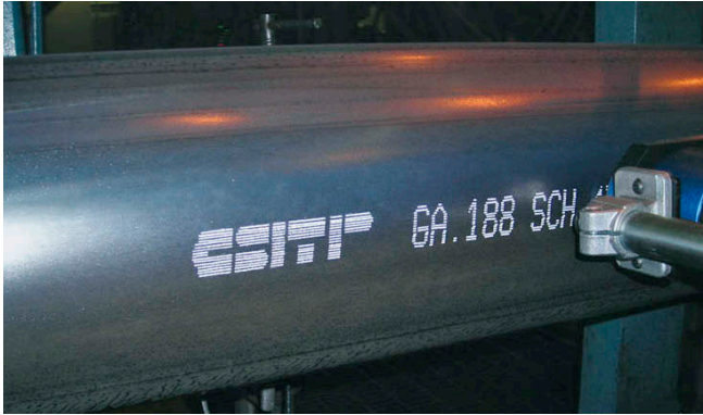
Marking of steel pipes
